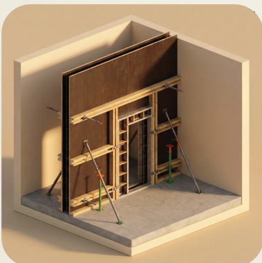
SHEAR WALL / LIFT CORE WALL
