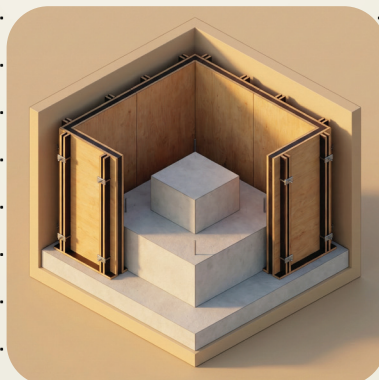
FOOTING + PEDESTAL FORMWORK
