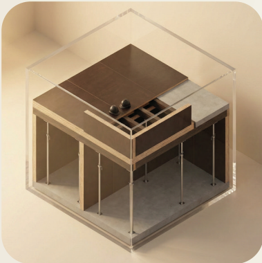
SLAB + BEAM FORMWORK BAY
